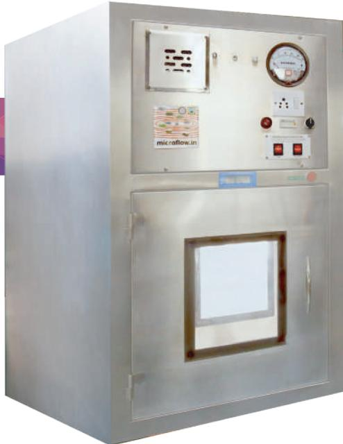
Clean room sterile dynamic pass through box is self contained units with class 100 laminar air flow unit installed at the entrance to the cleanrooms. The minimize the amount of particulate contamination entering the cleanroom by reduclng the operator traffic. The laminar flow in the pass box starts running, when the doors are opened for material transfer inorder to maintain air cleanlines required for the product.
